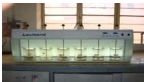
Picture (1) The jar test apparatus.
