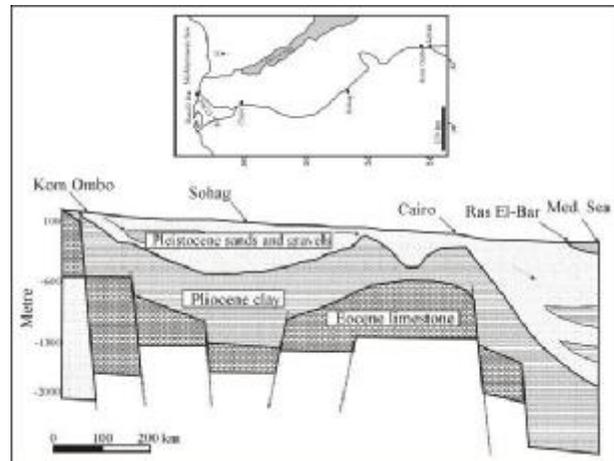
Fig. (2): Hydrogeological cross section along the Nile Valley
