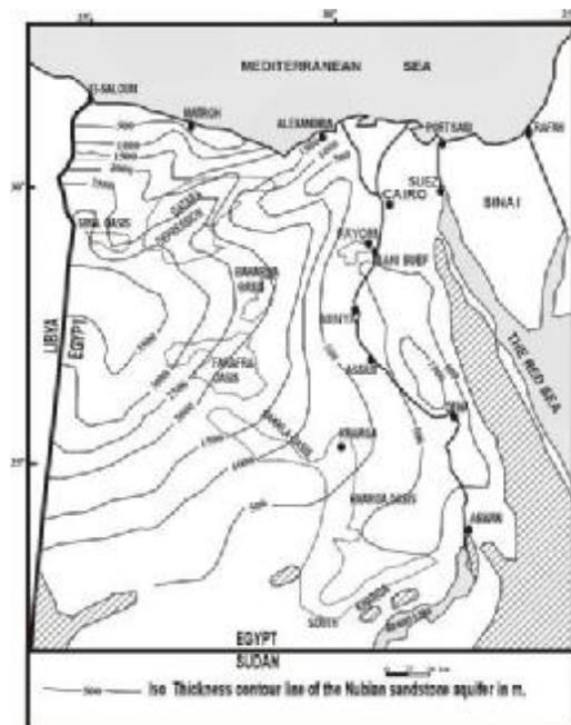
Fig. (4): Thickness of the Nubian sand stone aquifer in Egypt
