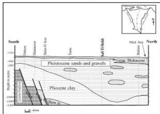
Fig. (3): Hydrogeological section along the Nile Delta
